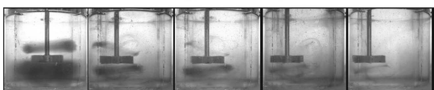
Fig. 6 Mixing process at different eccentric locations (FP)
